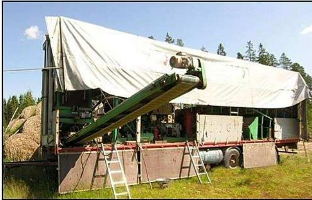
Ready pellet conveyor from pelletizing plant.
